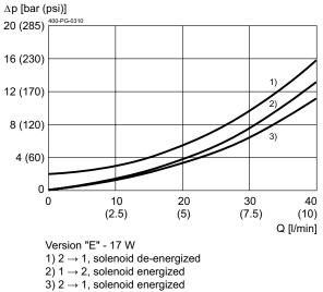
$\Delta p = f(Q)$  Pressure drop-flow rate characteristic
